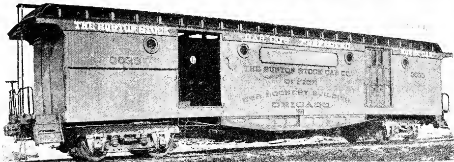
Fig. 45. STOCK CAR FOR HORSES AND PRIZE CATTLE. THE BURTON STOCK CAR COMPANY. Length, 44 ft. Capacity, 16 horses, or 22,400 lbs. (Interiors shown in Figs. 46 and 47.)
